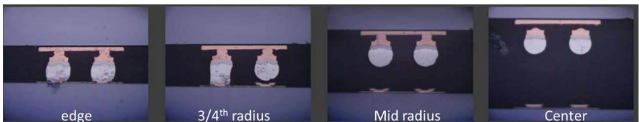
Figure 2.4.2: Mass reflow flip chip trial at BESI: evidence of deformation impact on electrical contact. For thermocompression, a bump shape similar to the “edge” bumps was set as reference.
