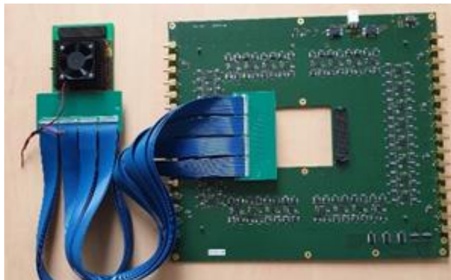
Figure 3.3.1: Electronic command card for the heating and beam phase shift of the OPA channels
