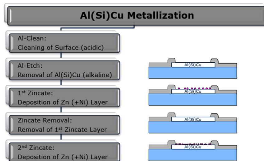
Figure 3: Pre-treatment of AlCu-Pad for following NiPPdAu- stack
