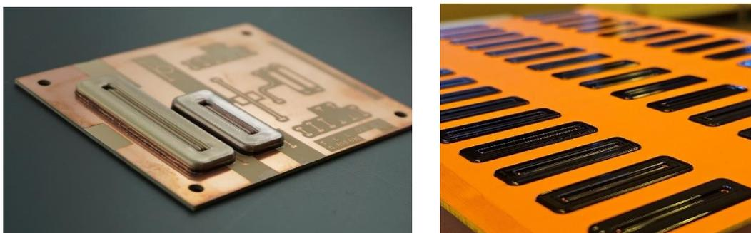
Figure 10: Metallized 3D waveguide antenna structure (left), high throughput production of waveguide antennas without metallization (right)
