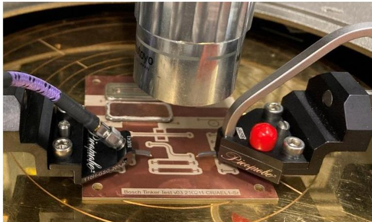
Figure 11.: The measurement setup: sample and OWP (on Wafer Probe)
