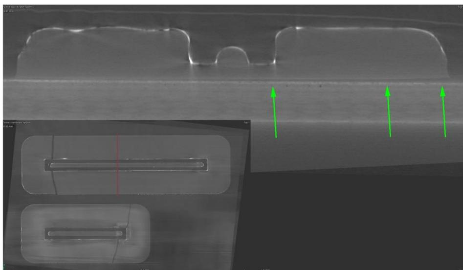
Figure 15.: The CT image of WG1 after the temperature cycling, clear signs of a delamination on the right side of the cross-section
