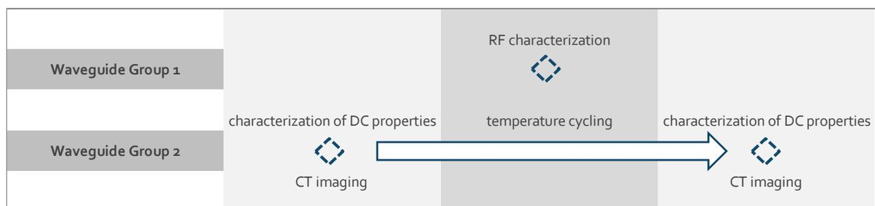
Figure 12.: Timeline of the evaluation of the waveguide samples
