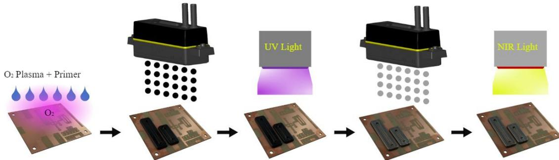
Figure 9: Fabrication process of metallized waveguide antenna structures
