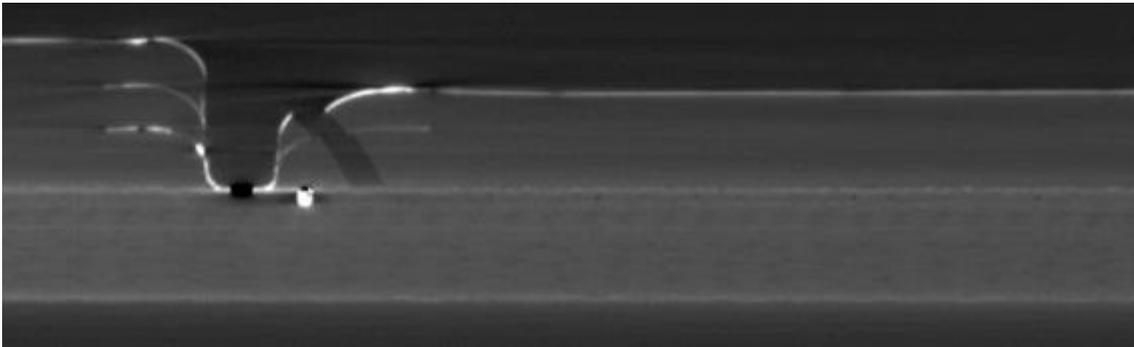
Figure 14.: The crack is visible on the left end of the waveguide channel of WG1
