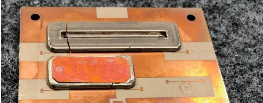
Figure 13.: Cracks are visible on WG1 and on WG2 as well.
