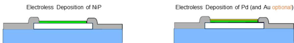
Figure 4: NiP and Pd electroless plating process steps
