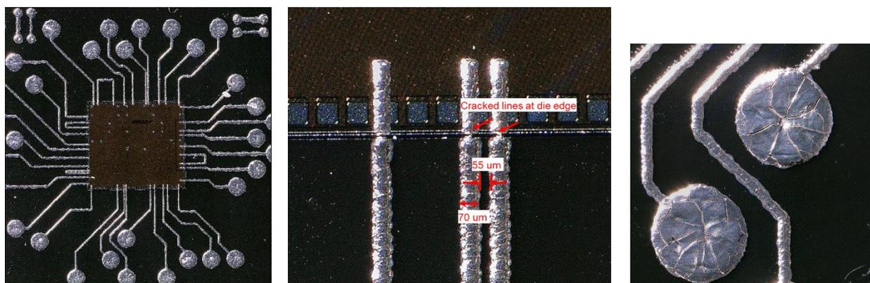
Figure 6: DC Layout on black imprinting material (left), all lines cracked at die edge (centre), large cracks on dog bone structures (right)
