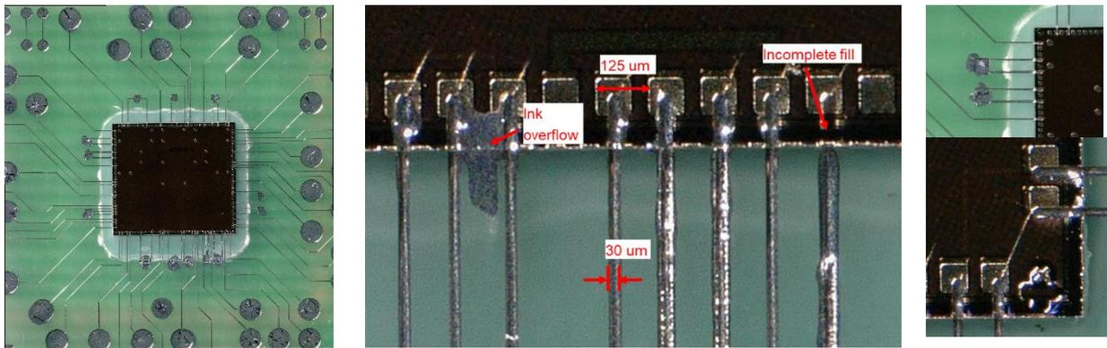
Figure 8: DC Layout on transparent imprinting material (left), ink overflow and incomplete fill at die edge (centre), overflow at printed bridges and misaligned lines (right)
