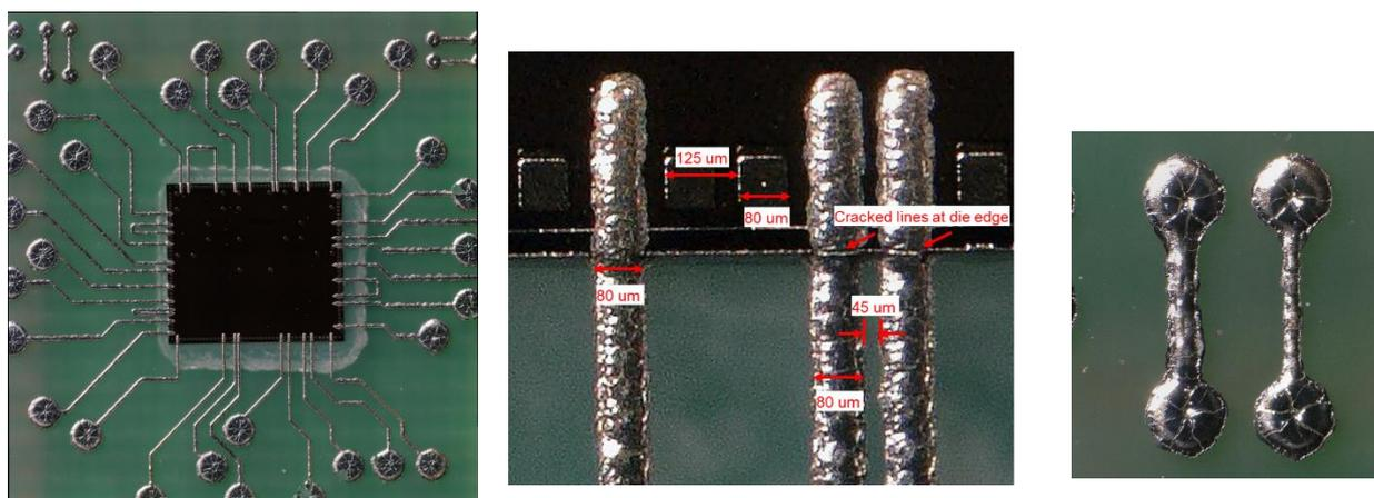
Figure 7: DC Layout on transparent imprinting material (left), some cracks around the microchip could be observed (centre), some cracks on dog bone structures (right)
