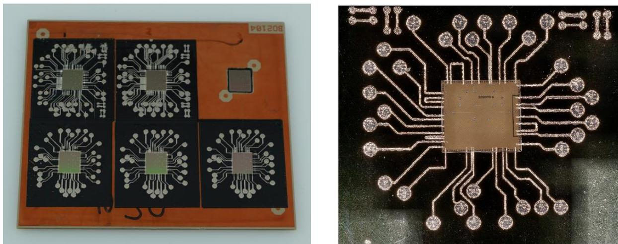
Figure 5: Example of process which was scaled-up to assemble, gap-fill and overprint (dielectric + conductive) 6 bare dies on one PCB carrier (left), detail of one bare die contacted via inkjet printing
