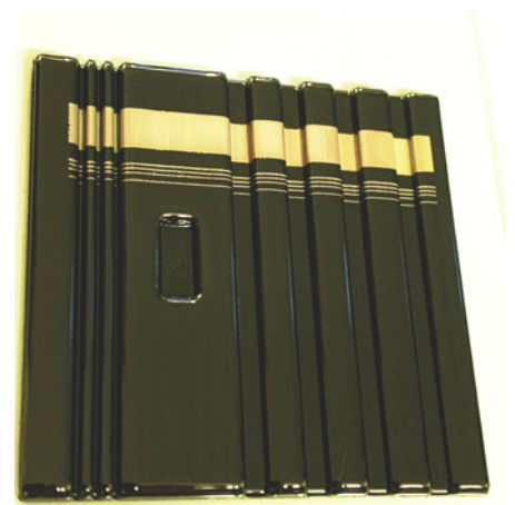
Fig. 3: Silver conductive ink printed on a 3D surface
