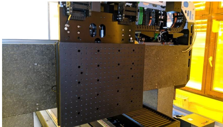
Figure 7: Image of second axis on which the laser sintering unit from Forth will be mounted for Laser processing inside the TINKER platform.
