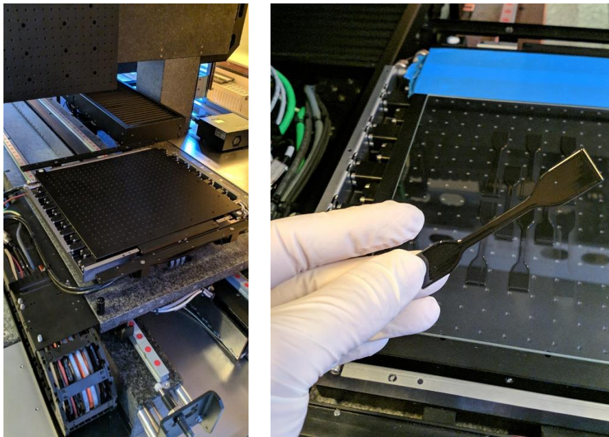
Figure 6: The image shows the print stage with high precision motor driven rotation correction capabilities. (right) In the upper right corner, the controller for the NIR lamp can also be seen. A 3D-printed dog-bone printed on the platform using UV-curable ink from Tiger (left).
