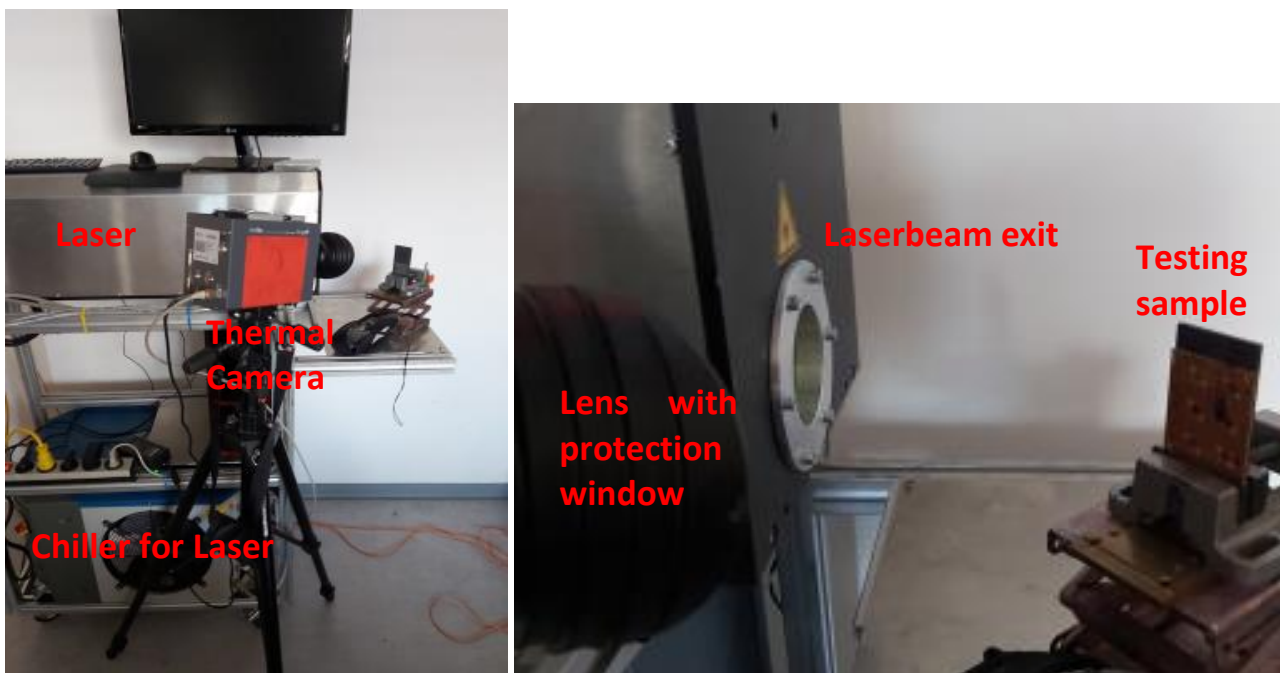
Figure 14: Photograph of testrig with laser, camera, and test sample.
